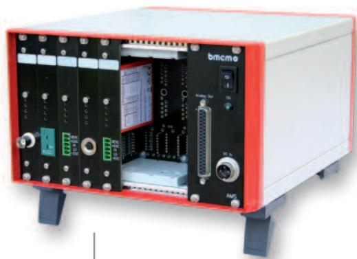
insert cassette in the plug-in position of the amplifier rack
